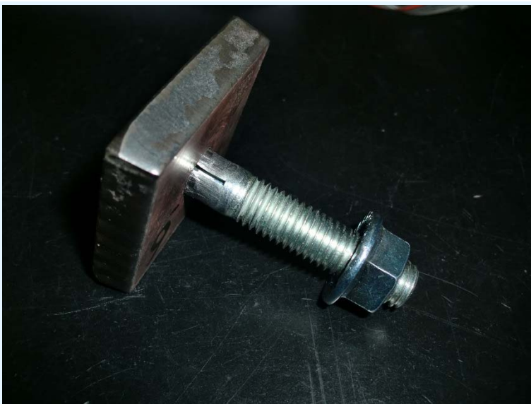
Figure 2.3 Complete tension test; pull-through
