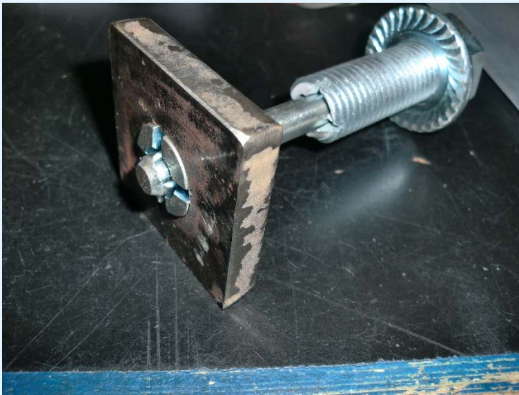
Figure 2.2 Completed tension test; fracture
