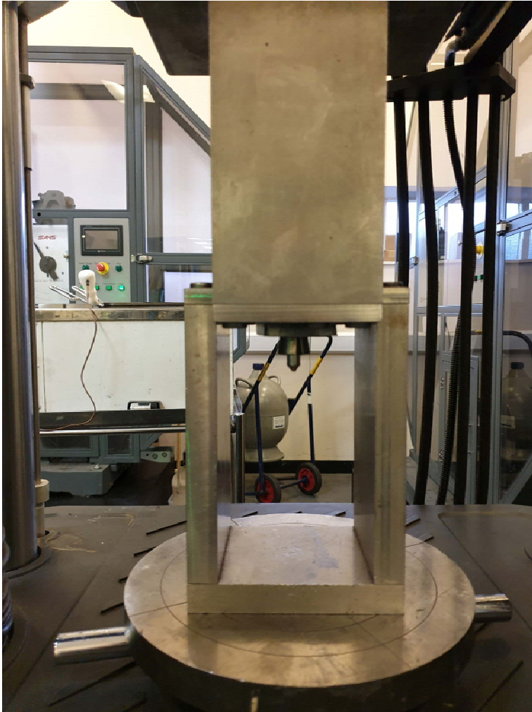
Figure 2.2 Tension test arrangement
