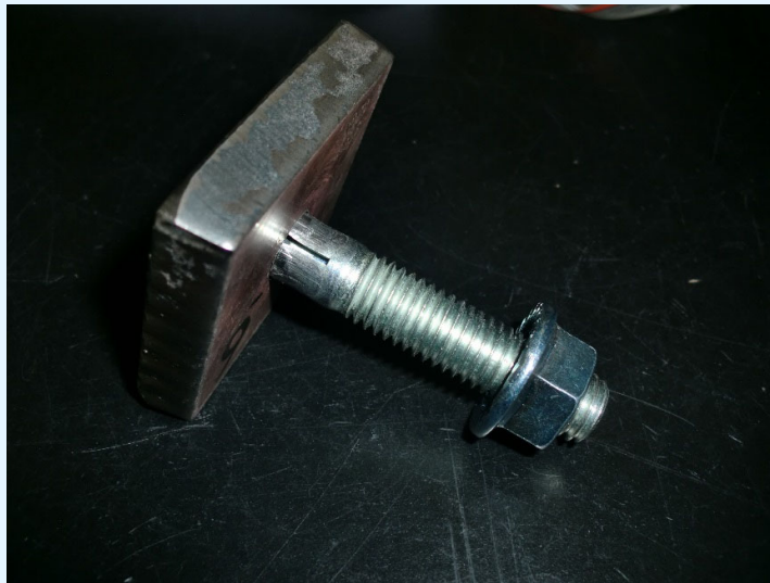
Figure 2.3 Complete tension test; pull-through
